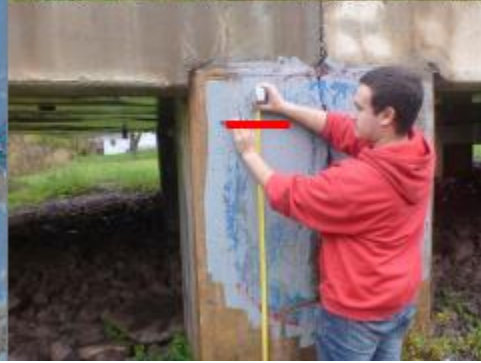
High water mark at the Trout River Bridge along Main Street; April 2014.
