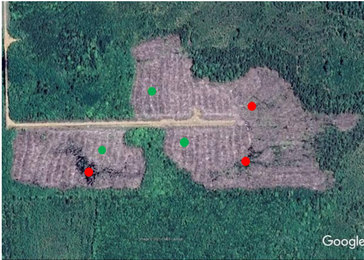
Figure 3. Further examples of the rutting and non-rutting points (indicated in red and green respectively). Image taken from the study area and points-enhanced in Microsoft word for illustrative purposes.
