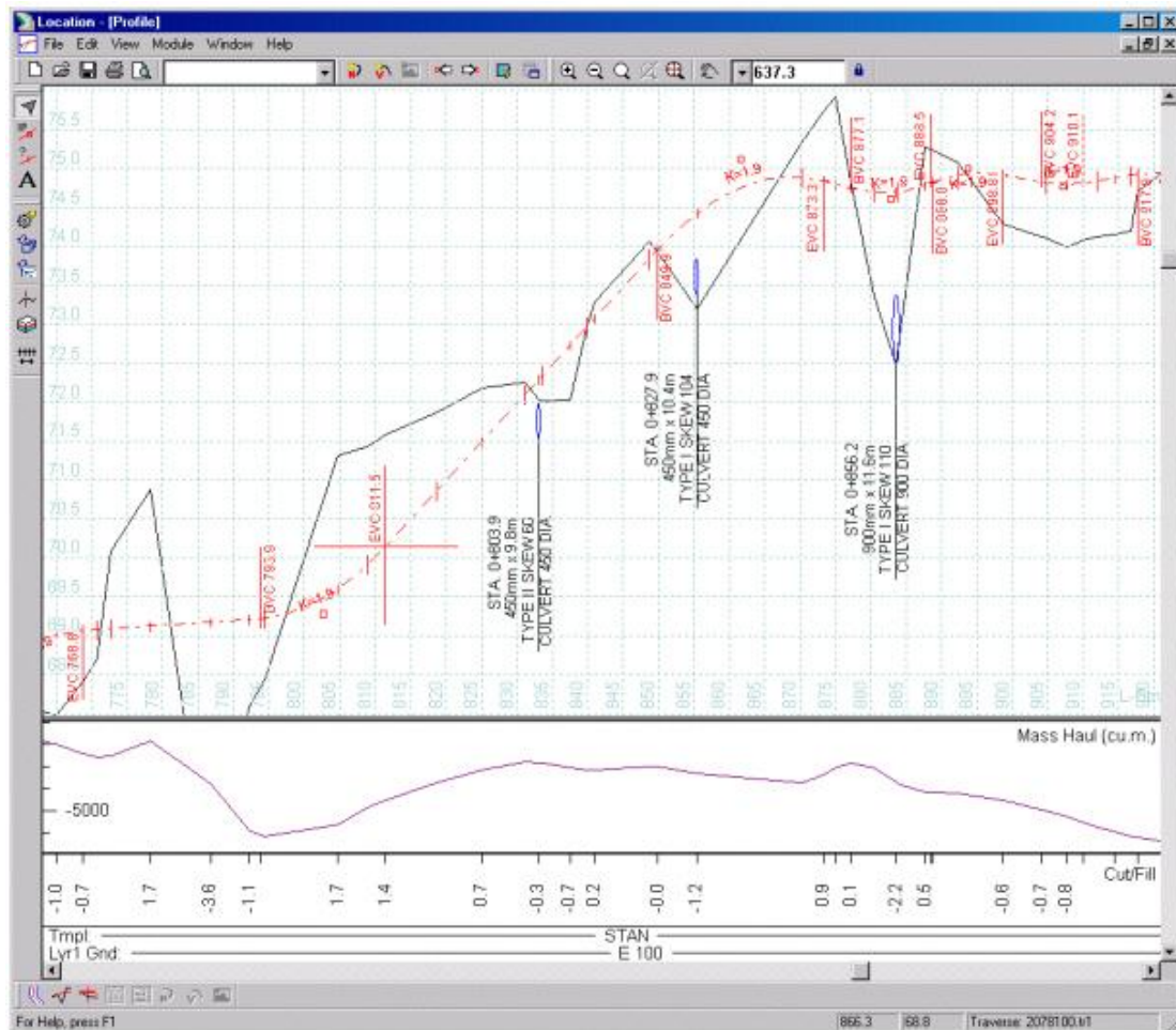
Figure 5.2g The output of RoadEng includes four kinds of road design information: plan, Profile, Cross Section, Data and Multi-Plot. This figure shows profile information produced by RoadEng program. ( http://www.softree-espanol.com/products/location_forest_pro.html ).
