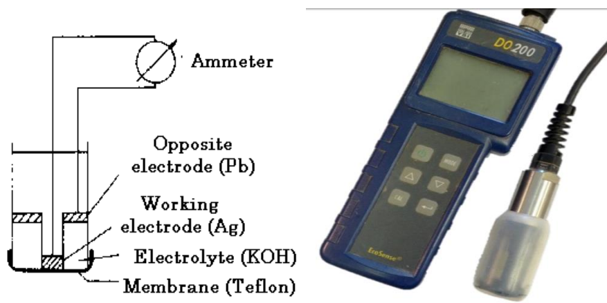
Figure 3. Structure and image of the DO probe.
