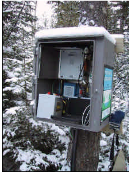
Fig. 4.3. Water quality monitoring station found in the Hayward Brook Watershed Study Area.
