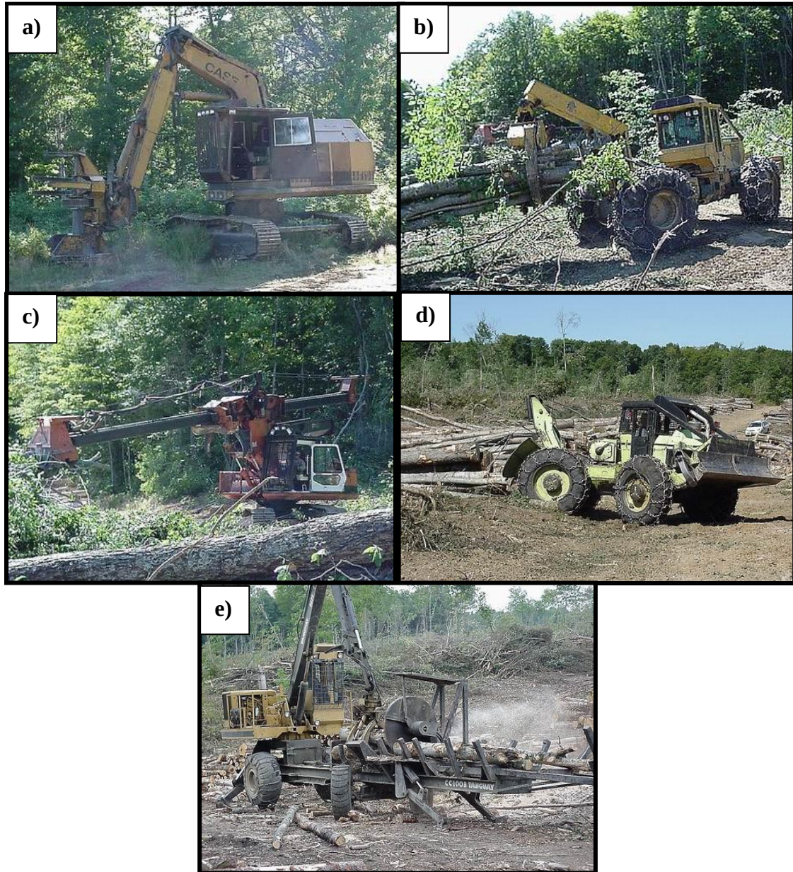
Fig. 3.11. Forest machinery used in the harvest of treatment catchments at Gounamitz Lake. Harvesting on the whole-tree catchment involved felling and piling of felled trees with a feller-buncher (a), movement to roadside with grapple skidders (b), delimbing with a delimber (c), and cutting to desired lengths with a slasher (e). Harvesting on the stem-only and extra-slash catchments involved felling and delimbing with chainsaws, movement of wood to roadside with cable skidders (d), and cutting of boles to desired lengths with a slasher.
