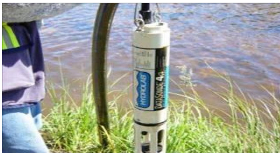
Figure 3.3 HydroLab Sonde 4A, with water quality sensors.
