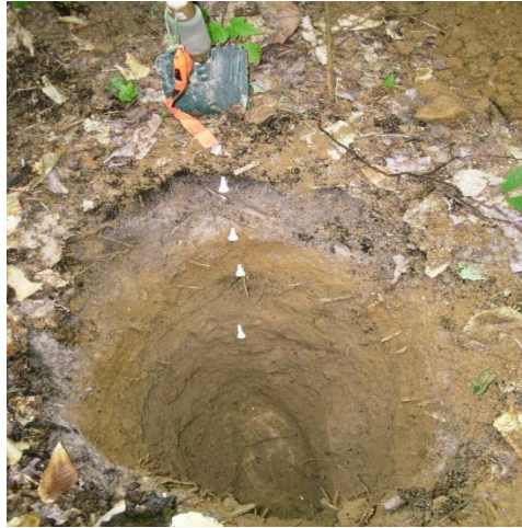
Figure 7. Photo of a soil pit showing golf tees used to mark horizons for soil survey.
