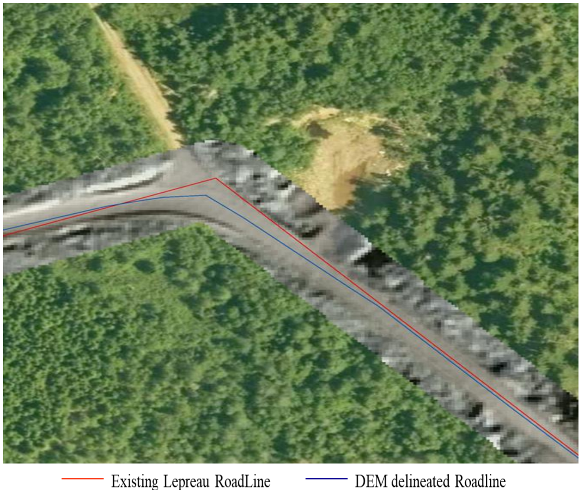
Figure 4.2. An example where the original road delineation veers off the elevated roadbed and falls into a ditch at an intersection along the road.
