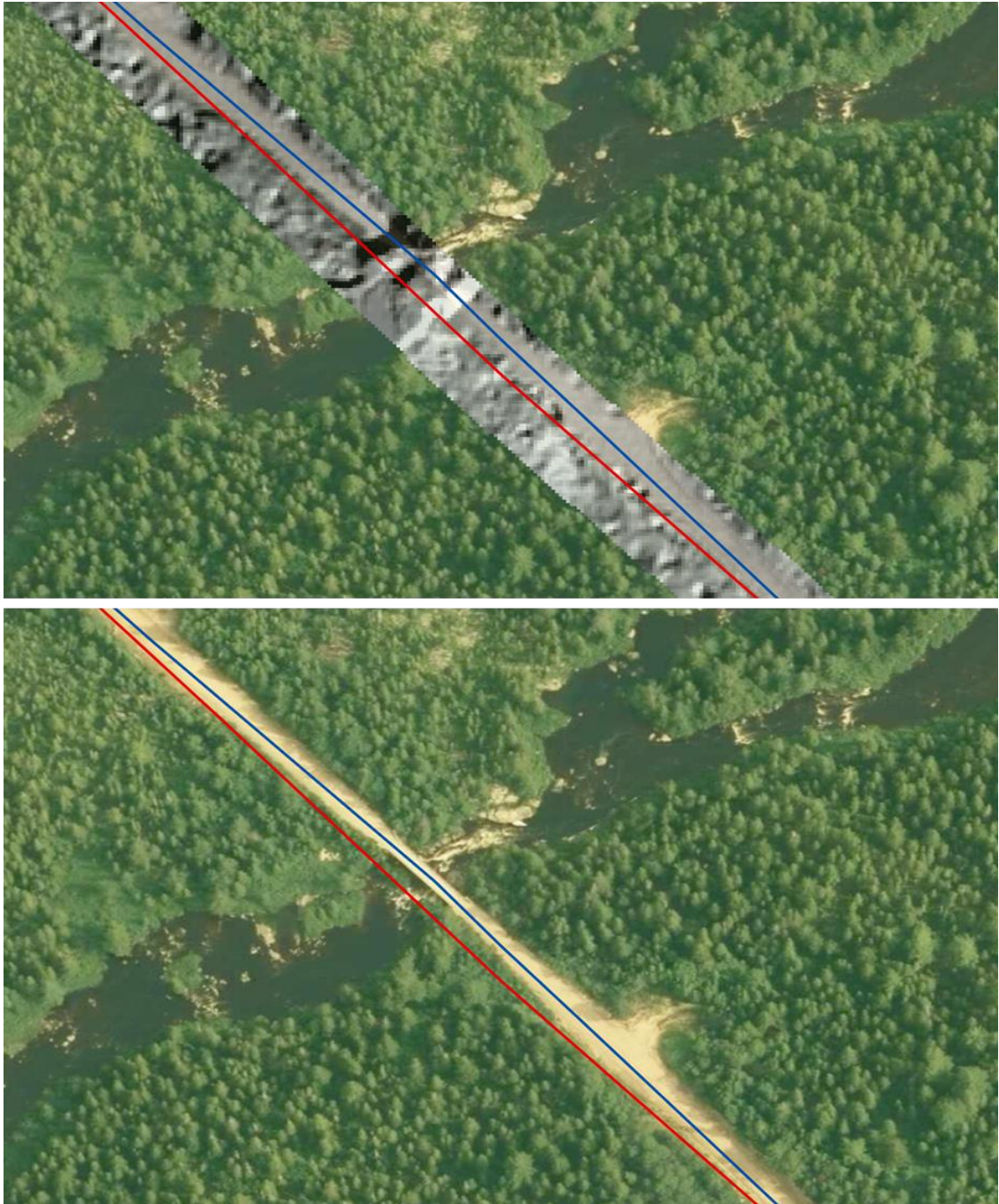
Figure 4.3. An example where the original road delineation veers off the elevated roadbed and falls into a ditch for about 200 m.
