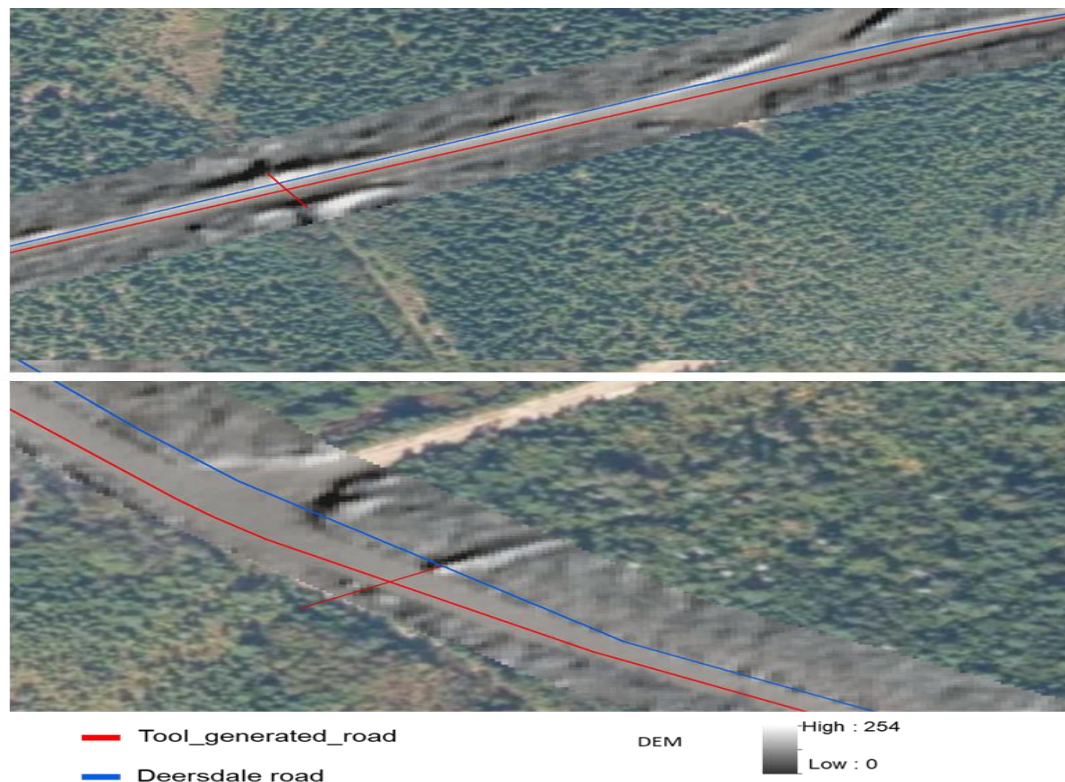
Figure 3.2. An example where the original road delineation veers off the elevated roadbed and falls into ditches along the road.
