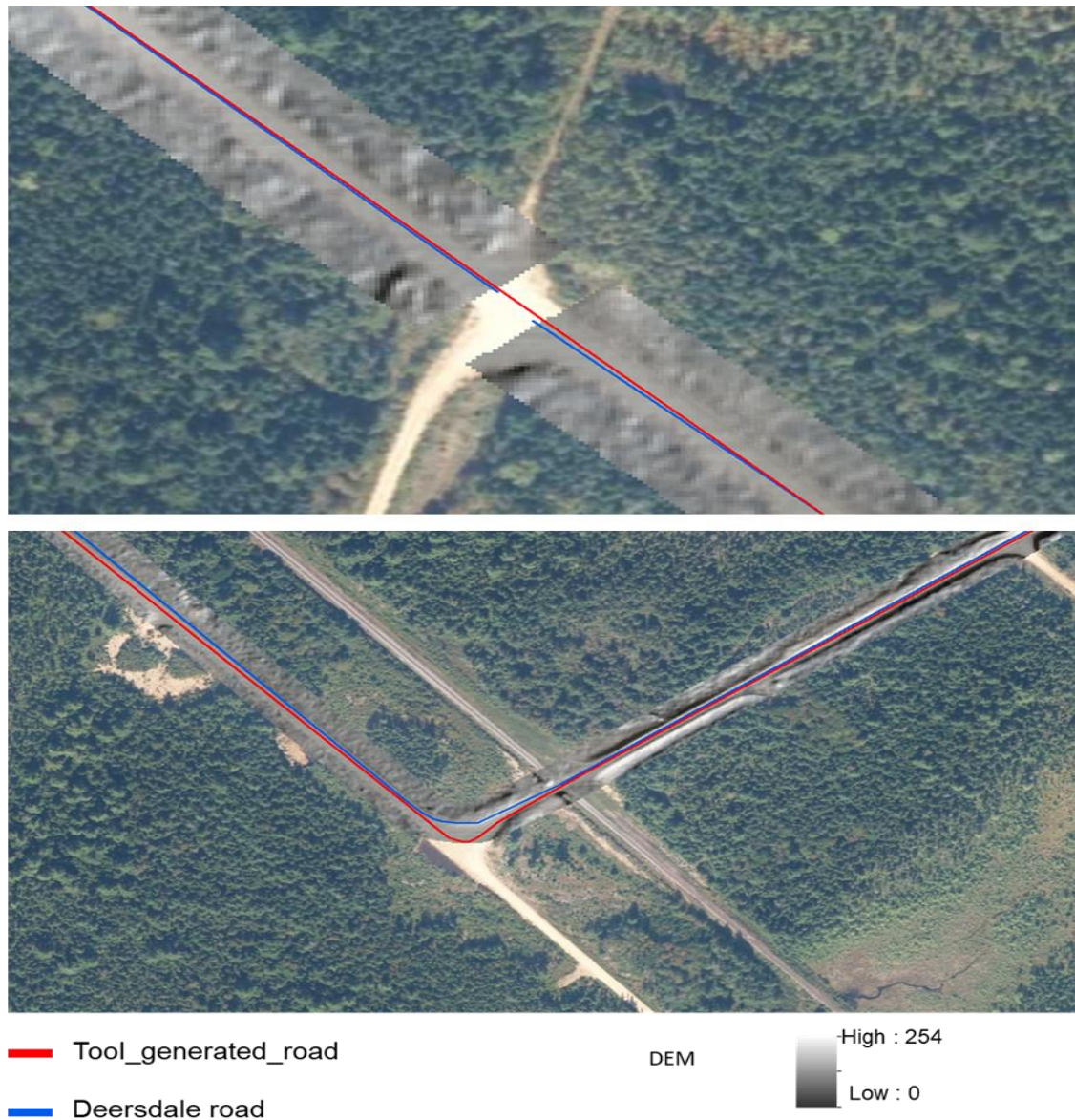
Figure 3.3. Two additional examples of where the original road delineation fails. Top: road line gap. Bottom: road line follows a ditch next to the road.
