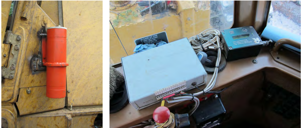
Figure 3.3: Ultrasonic distance sensor (left), datalogger box and inclinometer (right) installed in the Tigercat 635D.
