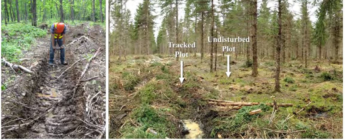
Figure 4.2: Penetrometer being used inside and outside forwarder tracks without brushmats.
